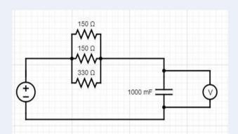
Supercapacitor Testing Schematic
