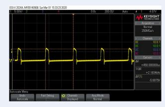
Direct measurement of voltage booster with 0.5V input
